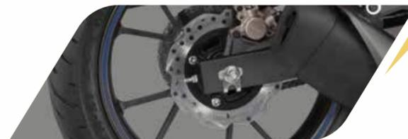
Get the utmost sense of control as you jirt with the wind. Because, with more power, comes the need to control it. Petal shaped discs help dissipate heat and maintain braking efficiency.
