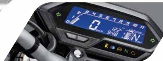
The perfectly positioned meter lets you know exactly how fast you're going as you assert your dominance. Be it night or day, see your info clearly with the 5-level Illumination Control on the crystal meter. Also, with the Gear Position Indicator, Battery Voltmeter and Service Due Indicator, stay above the rest. It also includes the Side Stand Indicator with Engine Cut Off that adds to the safety of the rider, indicating when the stand is down.
