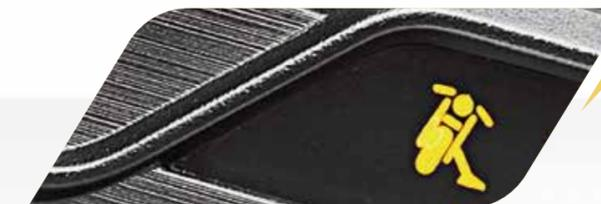
Adds to the safety of the rider. It cuts off the ignition if the vehicle is put in gear when the side stand is engaged.
