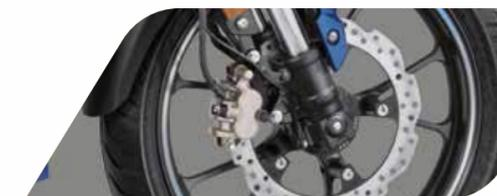
Braking is an integral part of biking. The ABS gives you better control as you brake, especially on slippery surfaces. By preventing the wheel from locking, it keeps you safe as you continue to fly against the wind.
